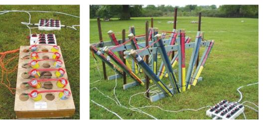
Electrical firing systems for fireworks displays Reproduced with kind permission from Mat Lawrence, MLE pyrotechnics Limited, www.mlepyrotechnics.co.uk (accessed November 2003).
